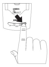
When the Mute indicator is selected, the unit is in Auto Mute Mode. In this mode you hear the full audio alert when a signal is first received. The audio alert automatically reduces to half volume for the duration of the warning.
